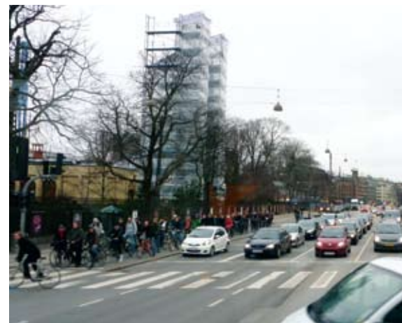
Fig. 3.83 Stop line for cars setting back from stop line for cyclists
