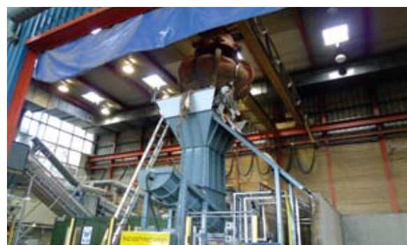
Fig. 3.48 Waste transferred to the rotating chamber
