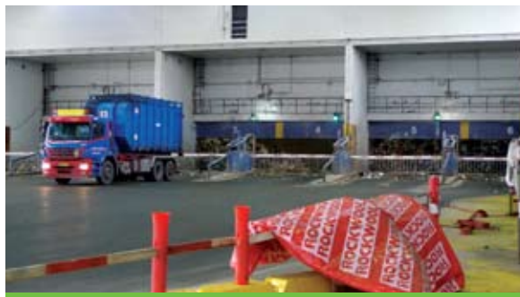
Fig. 3.45 Waste dumped into silo by truck
