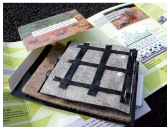
Fig. 3.76 Layers of material to facilitate vegetation and water-sealing
